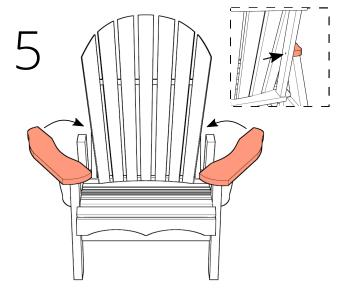
Match the key-holes on the arms onto the front legs. Make sure the arms are level on top of the legs before pivoting them 30° into place. Bolt the arms onto the back legs with 2 short bolts.
