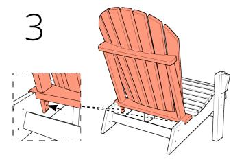
Slide the back into place and secure it to the seat using 2 short bolts.
