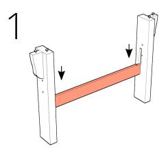
Insert the front leg support between the front legs, sliding it all the way down.
