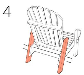
Attach the back legs to the seat using 4 long bolts.
